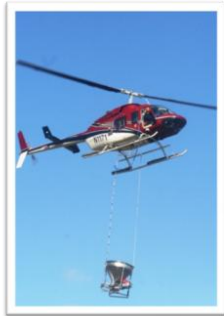
Figure 11. Aerial application of bait pellets from a spreader bucket slung beneath a helicopter.
