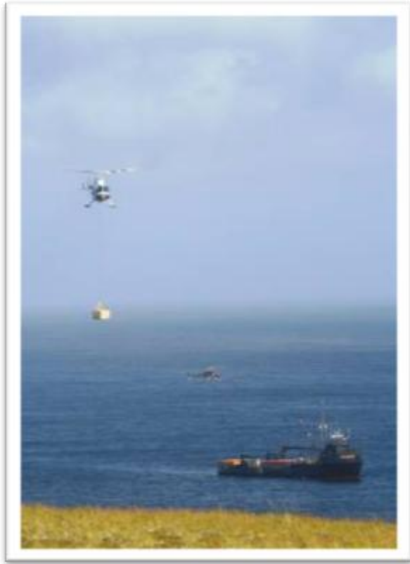
Figure 8. Helicopter slingloading BSV from aft deck of the M/V Reliance .
