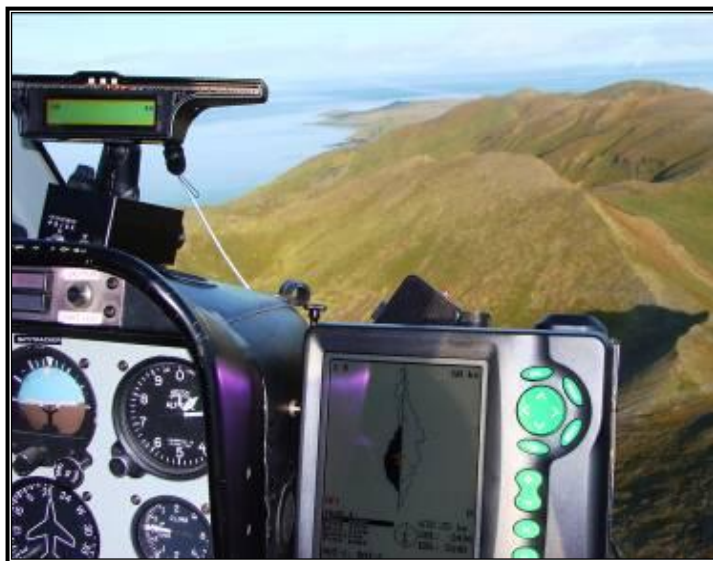
Figure 3. Onboard TracMap GPS used by helicopter pilots to monitor and guide aerial bait broadcast.
